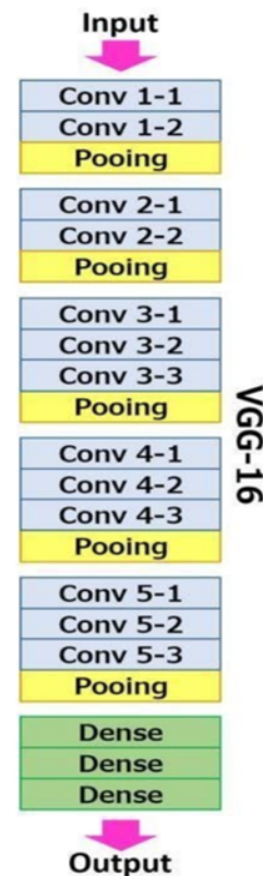
Figure 2. Architecture Of VGG – 16 Model
